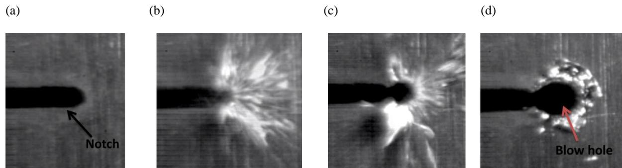
Fig. 1.2: (a-d) Time lapse photographs showing formation of a blow hole ahead of the notch tip in a conductor due to magnetic saw effect. The region near the notch vicinity is firstly, melted due to the Joule heating caused by excessive current crowding and subsequently, blown away by the electromagnetic forces, resulting in the formation of blow hole. (Ref: Gallo et al. Int. J. Fracture, 2011, vol. **167**(2): p. 183-193).
