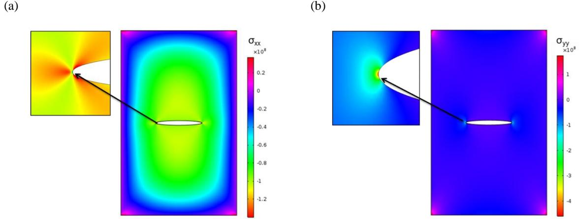
Fig. 1.3: FEM simulation showing the distribution of (a)  $\sigma_{xx}$  and (b)  $\sigma_{yy}$  in a thin conducting plate due to self-induced electromagnetic forces. Both  $\sigma_{xx}$  and  $\sigma_{yy}$  are compressive in the vicinity of the elliptical hole and try to close the crack.
