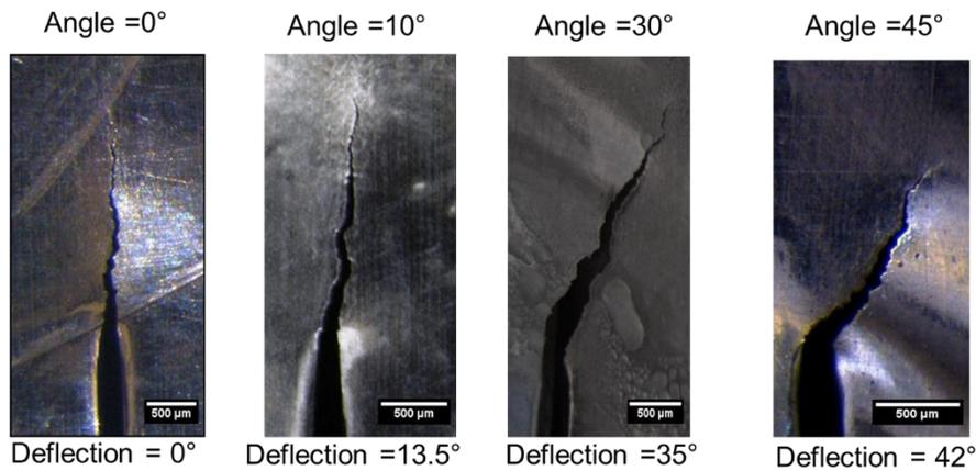
Fig. 1.6: Crack propagation under various mixed mode conditions due to the combined electric current and mechanical loading. The angle at top shows the angle at which mechanical load was applied relative to the mode I, whereas the deflection angle at the bottom shows the nominal angle at which the crack propagated relative to the original crack face.
