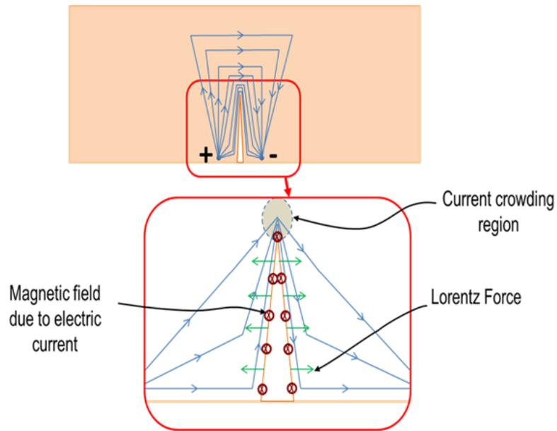
Fig. 1.1: Schematic illustration of reversal of electric current around an edge crack in a conductor upon application of a potential difference across the width of the crack. Electromagnetic force (or Lorentz force) induced due to interplay between electric current and self-induced magnetic field tries to open up the crack in mode I. Reversal of electric current around crack tip also causes current crowding in the vicinity of the crack tip which leads to Joule heating.
