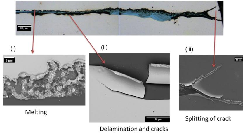
Fig. 1.7: Microstructural analysis of the failed edge cracked Cu thin film as observed under scanning electron microscope (SEM). SEM micrographs at different locations of the failed film show that the film failed by different mechanisms, such as (i) excessive melting, (ii) delamination and cracks (iii) splitting of cracks.
