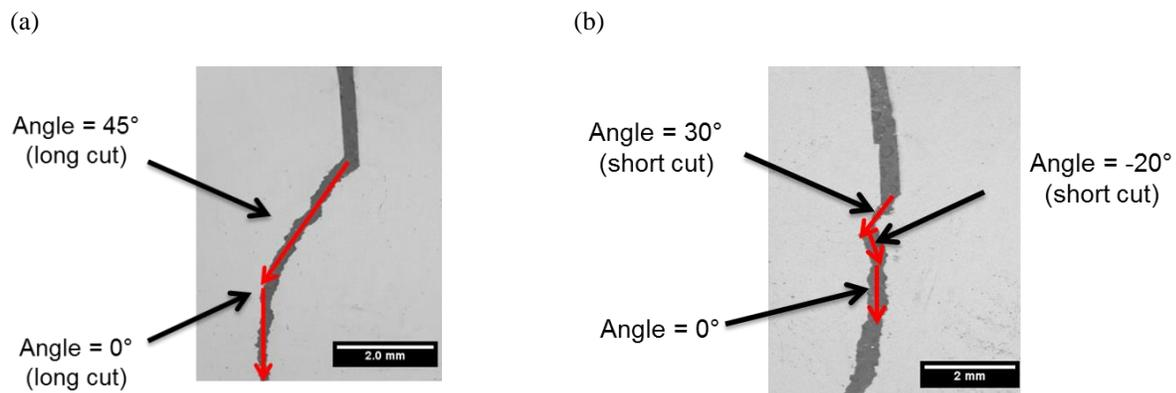
Fig. 1.8: Various shapes of cuts made in  $12 \mu\text{m}$  thick Al foil by manipulating mode-mixity during combined electromagnetic-mechanical fracture: (a) Longer cuts and (b) shorter cuts. Shape and size of the cut depend on the number of electric current pulses passed and the direction of mechanical load relative to the crack face.
