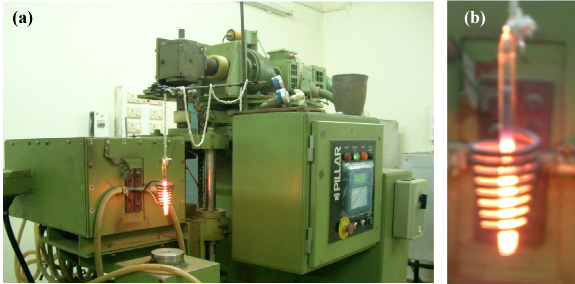
Figure 5.1: (a) The zone melting setup (make M/s Pillar India) used for directional solidification and (b) molten sample during the zone melting process.
