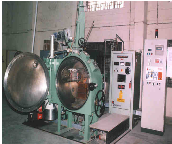
Figure 3.1: Vacuum induction melting furnace of the make of M/s Consarc, UK, used to prepare the alloys
