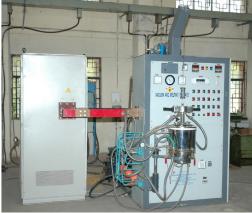
Figure 6.1: The vacuum arc melting furnace (male M/s Vacuum Technique), used for preparation of the alloy.
