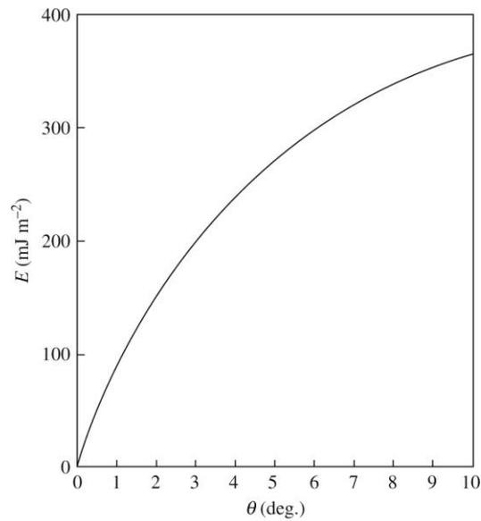
Example of the energy of a tilt boundary as a function of the tilt angle  $\theta$ .
