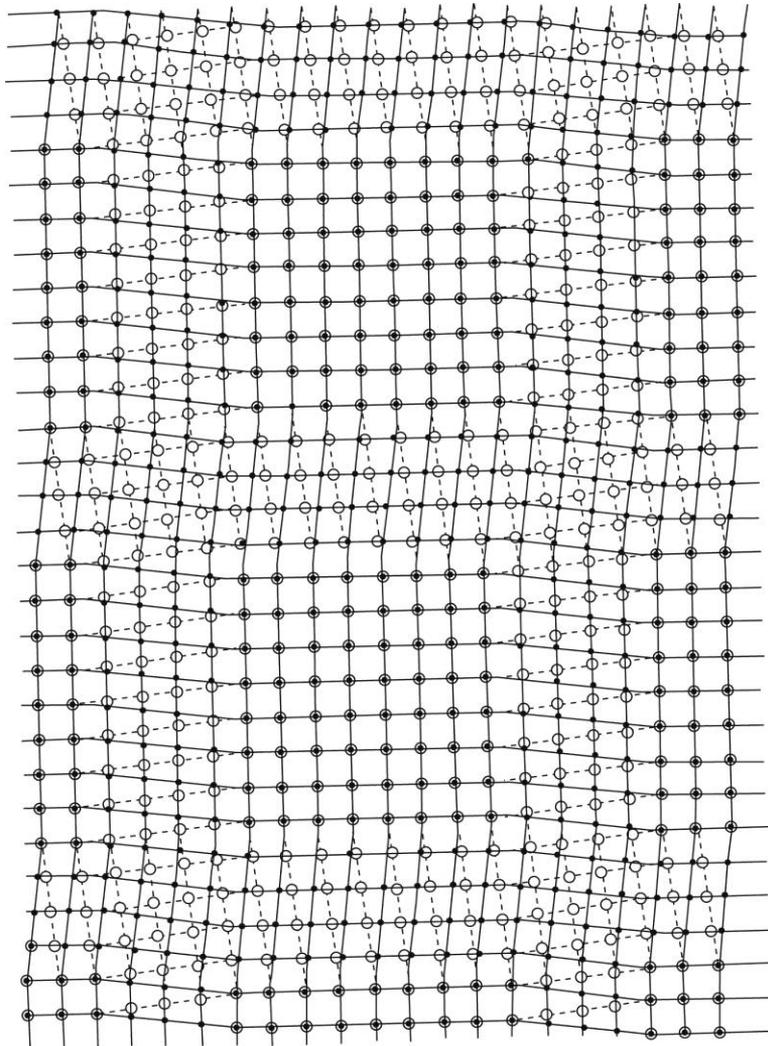
A low angle twist boundary in a simple cubic lattice.
