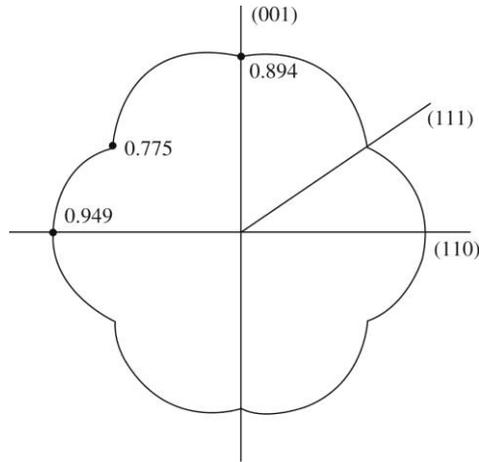
Possible  $(1\bar{1}0)$  section through the  $\gamma$ -plot of a c.c.p. metal. Values given are in units of the surface energy of a  $\{210\}$  surface (from J. K. Mackenzie *et al.* (1962)).
