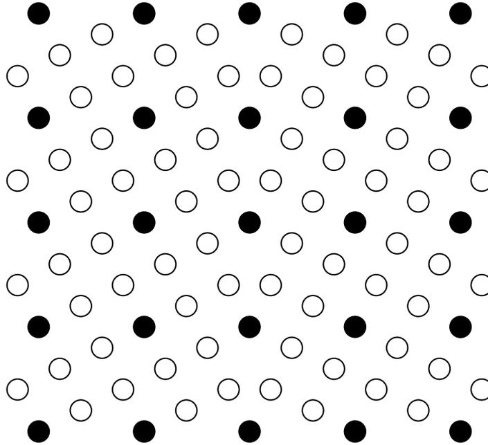
Schematic of a high angle tilt boundary of good fit between one grain on the left and one grain on the right in a simple cubic material. The boundary is normal to the plane of the figure. The dark circles represent atoms that lie on points of the lattices of both grains. Here,  $\Sigma$ , the ratio of the volumes of the primitive coincidence cell and the primitive crystal lattice unit cell, is 5.
