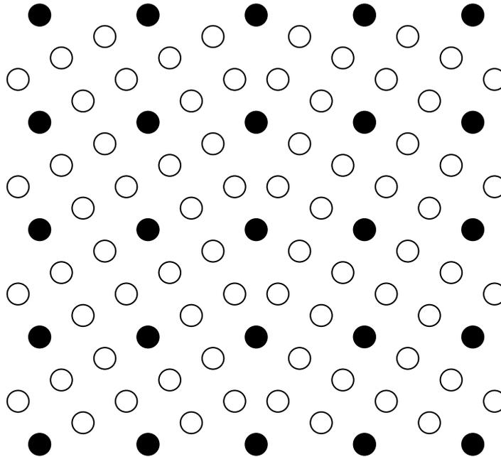
Schematic of a high angle tilt boundary of good fit between one grain on the left and one grain on the right in a simple cubic material. The boundary plane is vertical and normal to the plane of the figure. The dark circles represent atoms that lie on points of the lattices of both grains.
