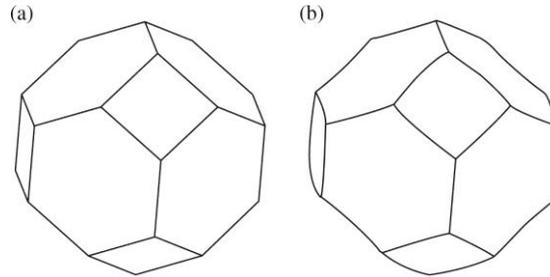
(a) Truncated octahedron and (b) distorted truncated octahedron which, when stacked, meets the requirement that the surface tensions balance at all junctions.
