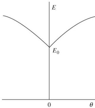
A schematic of energy  $E$  as a function of angle  $\theta$  away from a low-index plane
