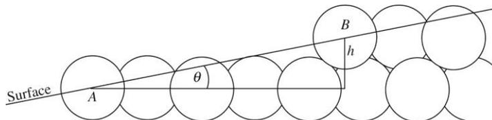
Surface at a small angle  $\theta$  to a {111} plane of a c.c.p. metal.
