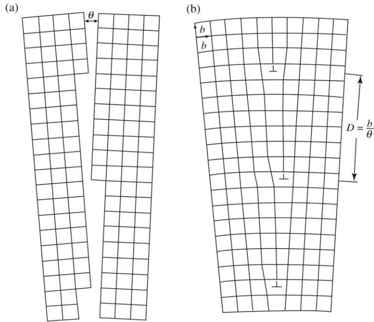
Low angle symmetrical tilt boundary in a simple cubic lattice.
