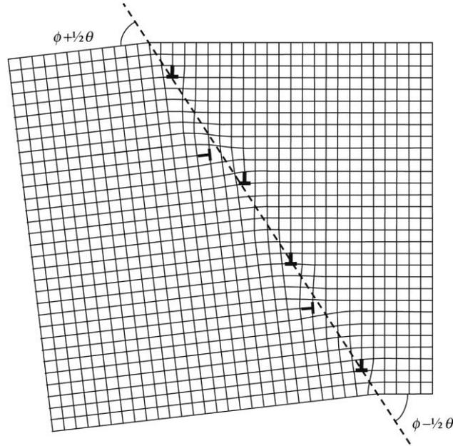
An asymmetrical tilt boundary in a simple cubic lattice where the misorientation across the boundary is  $\theta$ . The boundary makes an angle of  $90^\circ - \phi$  with the symmetrical tilt orientation
